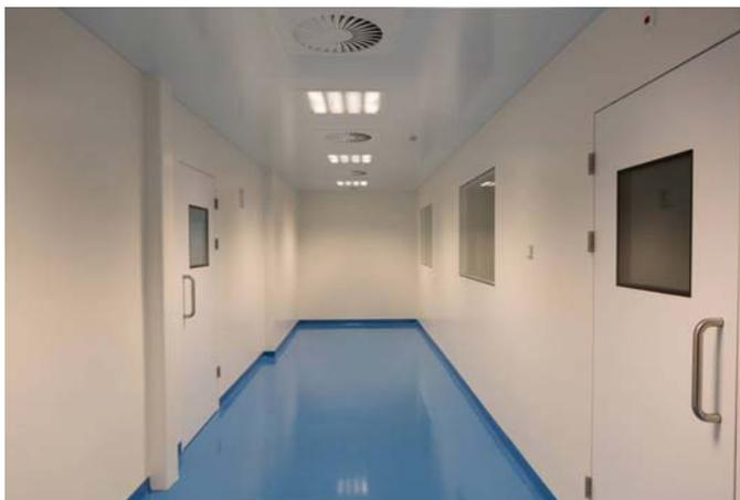
*Figure 7: The clean corridor as a distribution duct towards process rooms*
