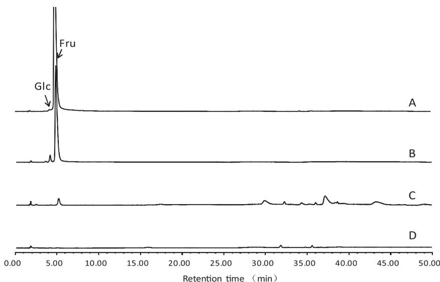
**Fig. 1.** HPAEC-PAD profiles of mono- and oligosaccharide products after treating *Erwinia* levan with (A) levanase and exoinulinase, (B) endoinulinase and exoinulinase, (C) levanase, and (D) no enzyme for 24 h. Levanase, exoinulinase, and endoinulinase were used at dosages of 400, 1000, and 400 U/g fructan, respectively. Labeled peaks are: Glc, glucose; and Fru, fructose. The peak was identified using authentic standard. The samples were of the same dilution and signal intensity scale.
