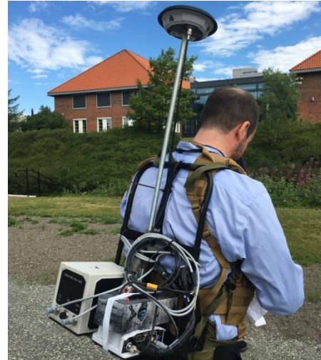
Figure 3: Rigid frame backpack holding ISA-100C based SPAN reference system.
