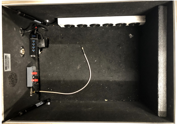
Fig. 1. RF shielded enclosure where training set measurements were performed.
