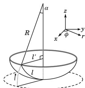
As shown on the left, when a flat wafer is bent on a spherical surface, an arbitrary circle with the radius  $l$  has to shorten down to  $l'$ . Therefore also its circumference has to change from  $2\pi l$  to  $2\pi l'$ . It can be shown that this *angular compression* causes a slowly varying strain component, that locally shifts the energy of the diffraction curve by
