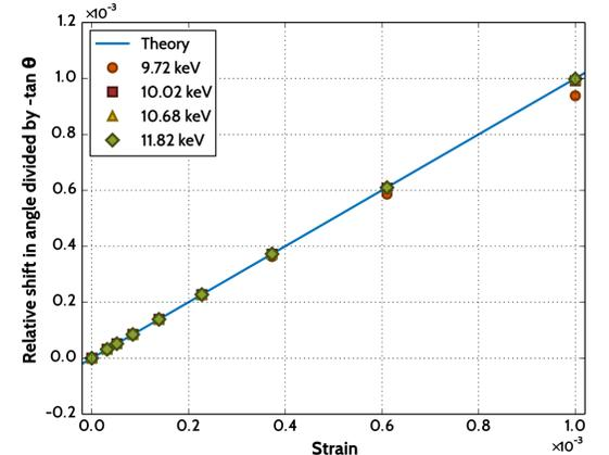
The validity of the derived shifts were tested by solving the TT-equations numerically with a Python code for Si(660) for constant strains up to 0.001. Apart from near-backscattering conditions where expression for  $\delta\theta$  ceases to be valid, the simulated diffraction curves look the same as for zero-strain case but with shifted  $\lambda$  and  $\theta$ , which agree well with the derived expressions.
