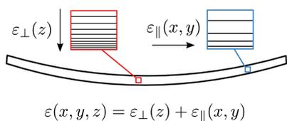
The diffraction curve of a large crystal can be calculated using the derived result if the strain field of the crystal can be separated into two components:
