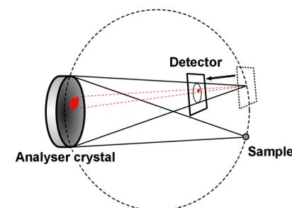
With a Johann-type spectrometer utilizing spherically bent analyser crystals, such a measurement can be performed with a position sensitive detector e.g. Maxipix.
