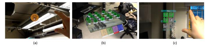
Fig. 10. Three basic AR interaction models: (a) The Floating Icons model, with the user gazing at the icon. (b) The WIM model in scale mode, with a hologram being engaged with. (c) The floating menu model, with three active items and three inactive items [171].
