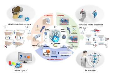
Fig. 9. The key principles of haptic devices that support user interaction with various tangible and virtual objects in the metaverse (Image source from [167]).
