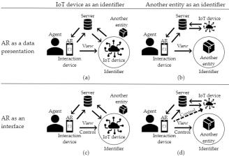
Fig. 12. Four interaction models proposed in [182], categorised by whether an agent can control the IoT device through AR (c,d) or not (a,b), and whether an IoT device (a,c) or another entity (b,d) functions as an AR identifier.
