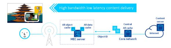
Fig. 20. An example MEC solution for AR applications [454].
