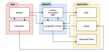
Fig. 22. Network- and User-aware applications in the metaverse. A synergy between the traditional network layers and the application-level measures of user experience allow for maximising the user experience given the actual network conditions.
