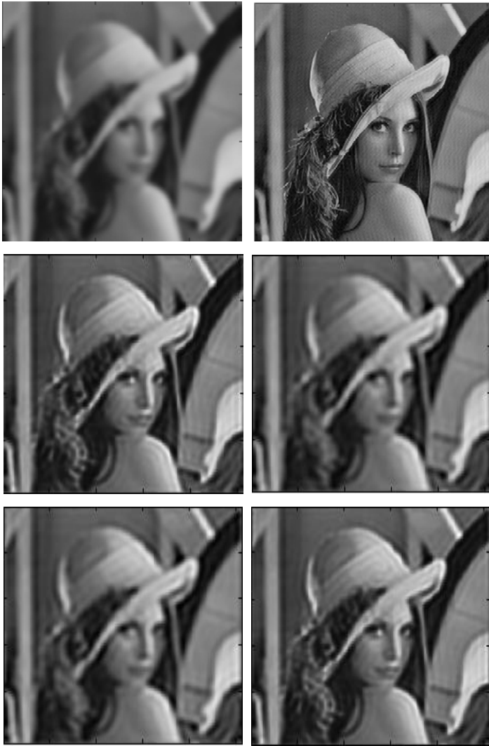
Fig. 6. Blurred images (top left), restored using the proposed method (top right), Richardson Lucy (middle left), regularised filter (middle right), Wiener Filter (bottom left) and blind Richardson Lucy method (bottom right).
