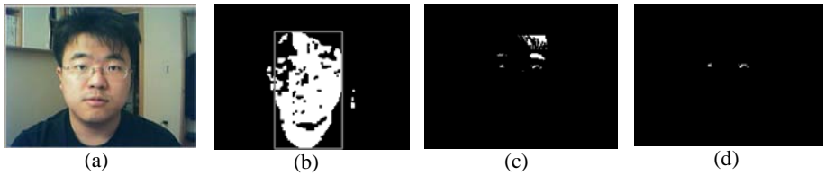
Fig. 5. An example of eye detection. (a) a original image, (b) the extracted facial regions (c) the classified image by the neural network, (d) the detected eye region after post-processing.
