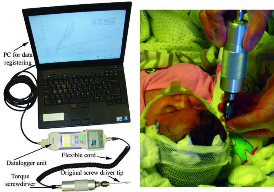
Fig. 2. Measurement set-up. Left: high-resolution digital torque screwdriver connected to a conventional laptop. Right: measurement of torque during distraction.
